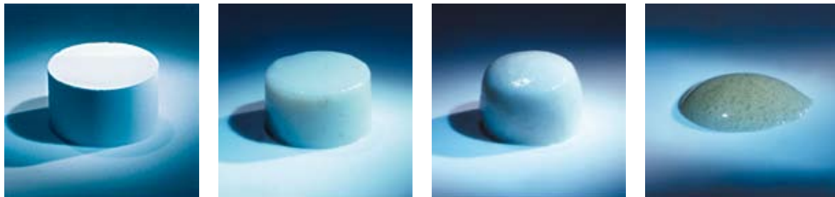
Different flow characteristics of bonds at the same firing temperature
